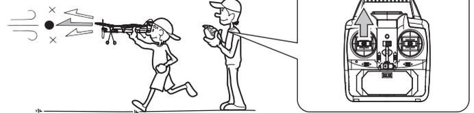
2. Apply 3/4 throttle while facing into the wind. Hold the plane horizontally and launch straight and level with a gentle pushing motion.
